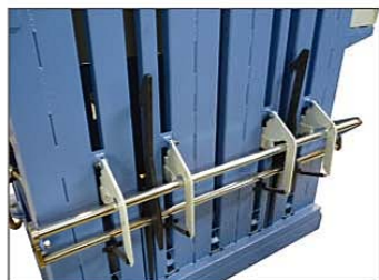
開門上升自動排出與止逆裝置裝置 Auto hook in while open door for eject and topper device
